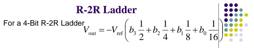
For general n-Bit R-2R Ladder or Binary Weighted Resister DAC
